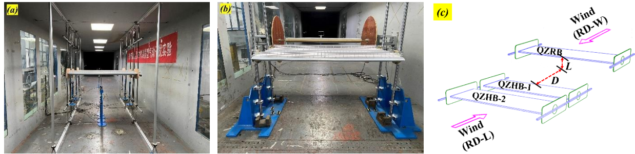
Figure 2. Photos and schematic diagram of wind tunnel tests: (a) vibration-measurement test; (b) force-measurement test; (c) schematic diagram.
